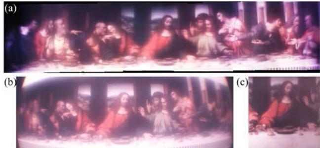
Figure 6: Wide-angle imaging comparison. Image of ‘Last Supper’ by (a) our device, (b) a fisheye lens, and (c) a solid lens. The three lenses had the same aperture.
