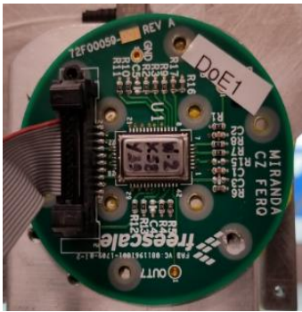
Figure 11: Board-mounted in-frame package for evaluation of QCU differential voltages of engineering samples.
