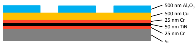
Figure 1: Substrate seed layers with lithographically patterned alumina electroplating mask.
