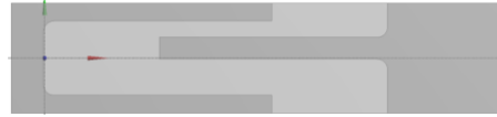
Figure 1: Conventional Quadrature Compensation Unit (Type A) Structure Design with biased electrostatic gap
