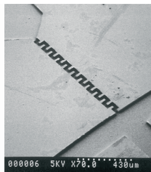
Figure 3: Scanning electron micrograph of the mixing region.
