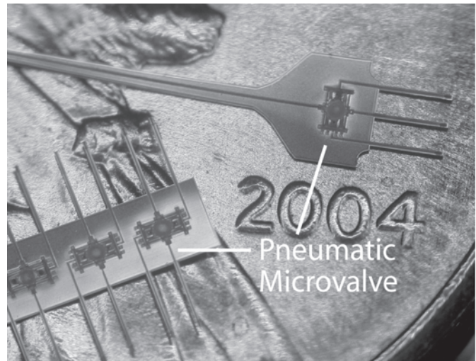
Figure 1. A drug delivery probe with integrated microvalves
