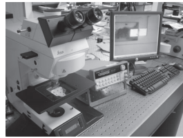
Fig 7. Experimental setup with a Leica DMRXA2 upright microscope, and Leica 350fx CCD camera.
