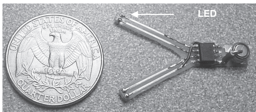
Figure 5. Circuit board with a miniature LED based device to regulate direction of flight in the adult moth.
