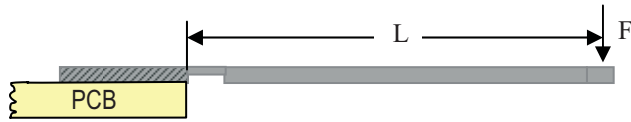
FIGURE 2: Side view of the sensor with 'L' being the length between the point where force F is applied and the anchor.
