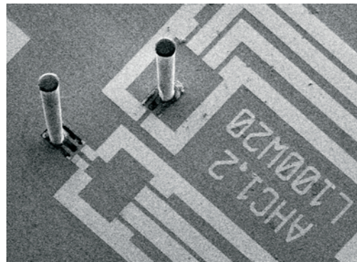
Figure 11. A pair of AHC sensors oriented orthogonally for resolving angular flow information.
