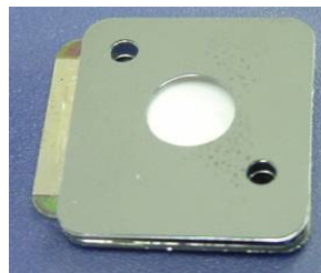
Figure 1. A photograph of a Si microfabricated vapor-fed fuel cell (Si- \mu VFFC). The MEA and the Si wicking structures are bonded temporarily with a PDMS membrane.
