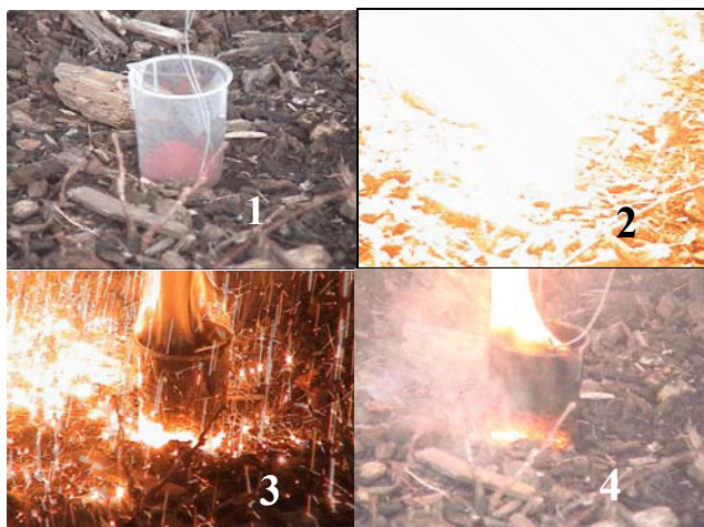
Figure 9. Micro Glow Plug igniting 5 grams of thermite in a plastic beaker.
