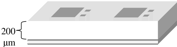
Fig. 6 PDMS cast in the SU-8 mold with vertical microchannels. The large reservoir is 500 \mu\text{m} x 500 \mu\text{m} while the two smaller capillary channels are 100 \mu\text{m} x 100 \mu\text{m} . The small capillaries are separated by 100 \mu\text{m} from each other, and from the large reservoir.
