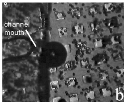
Figure 8: Channels isolate electrodes/electrolyte from foreign particles in surrounding medium. Chips pre-filled with 1M phosphate buffer were immersed in water containing 10 \mu m beads. Any beads that entered the channel were trapped by the gas-liquid interface formed by exiting bubbles; additionally, the liquid motion caused by the exiting bubble aggregated nearby beads at a distance approximately equal to the exiting bubble diameter.
