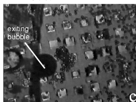
Figure 8: Channels isolate electrodes/electrolyte from foreign particles in surrounding medium. Chips pre-filled with 1M phosphate buffer were immersed in water containing 10 \mu m beads. Any beads that entered the channel were trapped by the gas-liquid interface formed by exiting bubbles; additionally, the liquid motion caused by the exiting bubble aggregated nearby beads at a distance approximately equal to the exiting bubble diameter.
