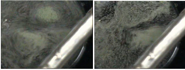
Fig. 9 Liquid trace changes when the RF frequency is changed by a small amount.
