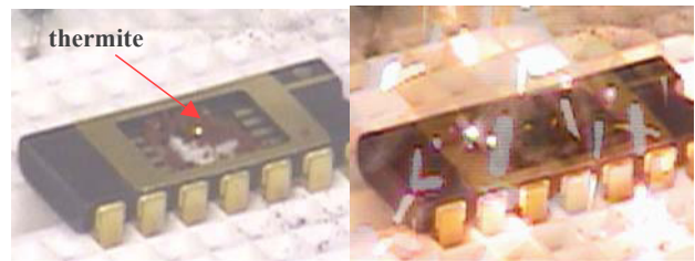
Figure 7. Chip-scale thermite reaction initiated by Micro Glow Plug. (a) MGP starting to glow, (b) ignition! The sequence took about 200 msec.
