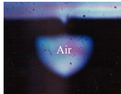
Figure 4. Optical image of visible light propagating through roughly 6 millimeters of a miniature Bragg fiber. The magnification is 1000 times. The Bragg fiber was targeted to have a lower wavelength cutoff at 400nm. The mirror stack consisted of SiN and SiO 2 .
