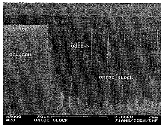
Figure 3. SEM image of the cross section of a 30- \mu\text{m} -deep sacrificial silicon-oxide block.
