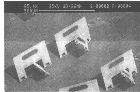
Figure 11. SEM micrograph of an array of 3-D devices. H_{ext} has been removed.
