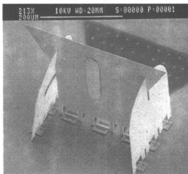
Figure 9. An SEM micrograph of a 3-D device using three Type I flaps. The sequence of actuation is not critical to the assembly of this device.
