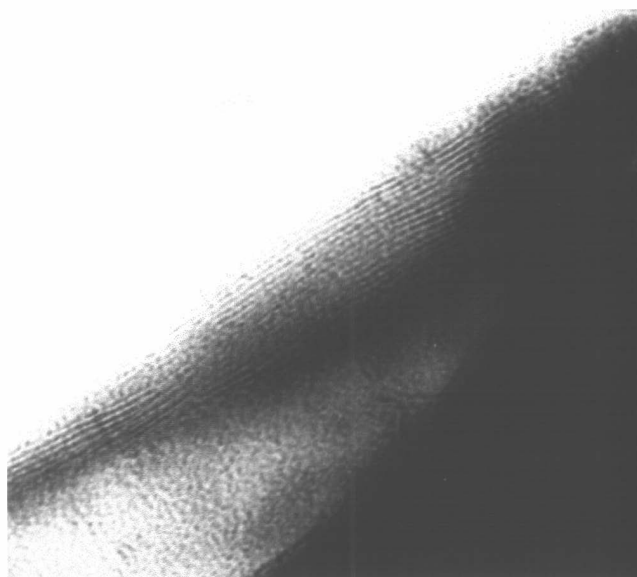
Figure 5. TEM of laser deposited Nb-TMS1 film.
