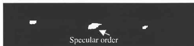
Figure 5. Diffraction pattern of the blazed grating. Diffraction orders not adjacent to the specular order are very small compared to the specular order.
