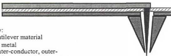
Figure 1. Schematic layout of combined SFM/coaxial tip with a coplanar waveguide running along the cantilever.
