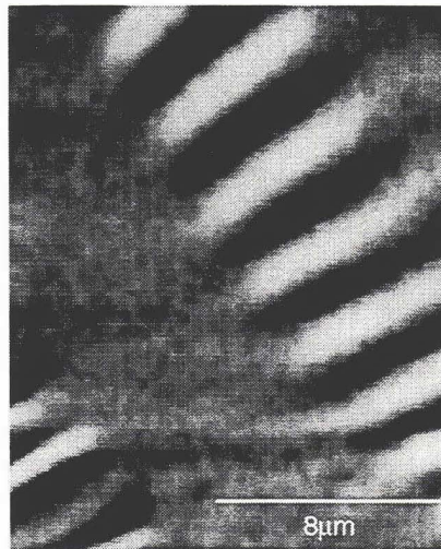
Figure 10: Imaged 8 \mu\text{m} wide disk drive track.
