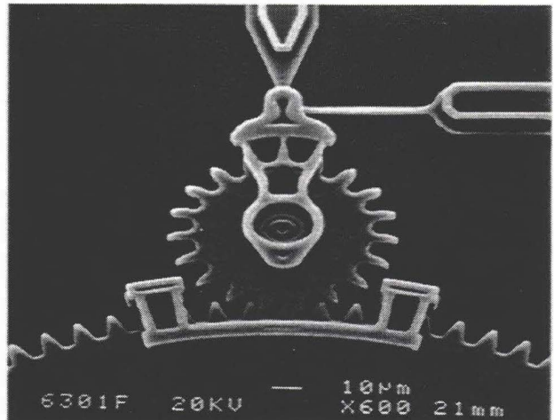
Figure 5. SEM of second-generation tooth design. The drive gear pitch circle radius is increased from 26 \mu\text{m} to 38 \mu\text{m} to accommodate the deeper tooth design and additional teeth. Note the deeper and multiple tooth engagement relative to the gears in Figure 1.
