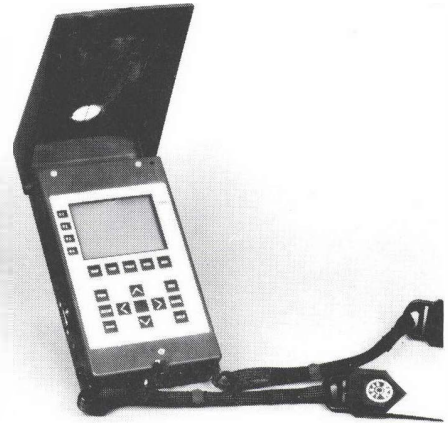
Figure 1. Personal Navigator System Containing Solid-State Compass
