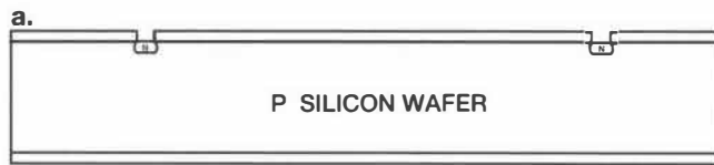
Pattern oxide for N-diffusion & backside alignment marks
