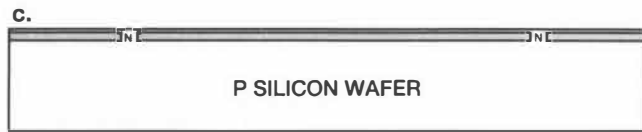
Anneal to form buried oxide
