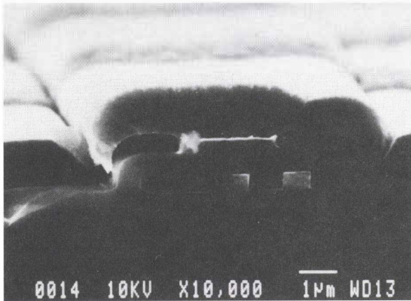
Fig. 5: Attack of the silicon substrate due to inadequate step coverage of PECVD films.
