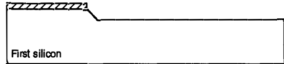
1) KOH recess to define capacitor gap.
